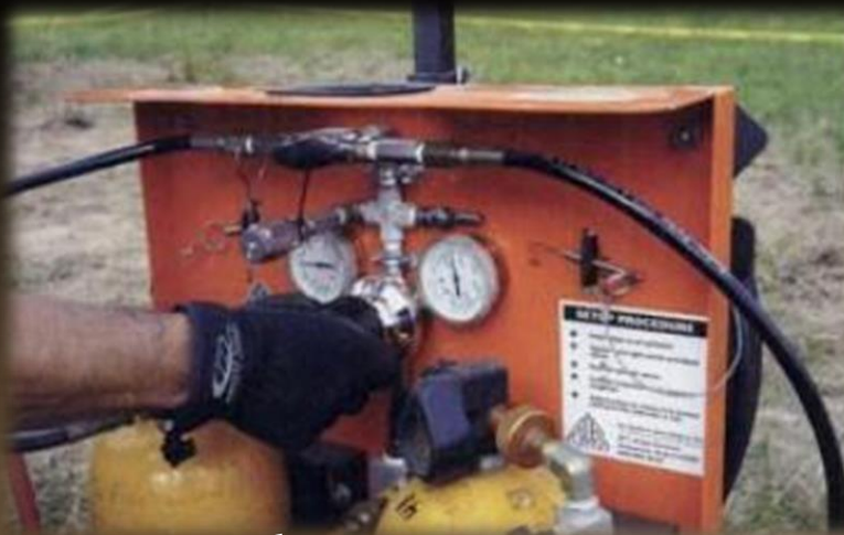
Attach Air System to Strut 116 psi. for Airshore Trench
