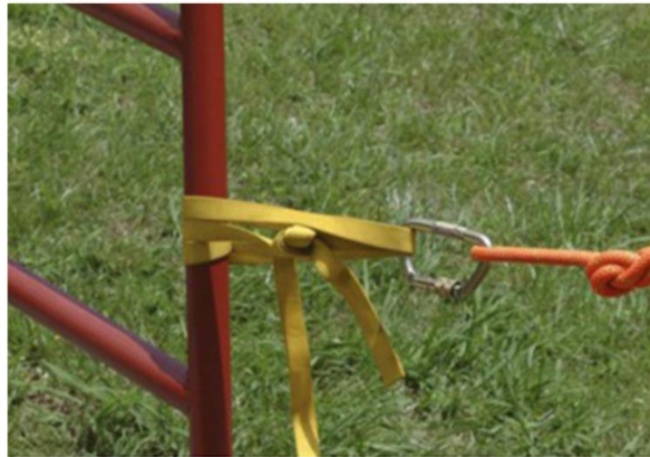
Multi-Wrapped web Sling 3 Bight Anchor
