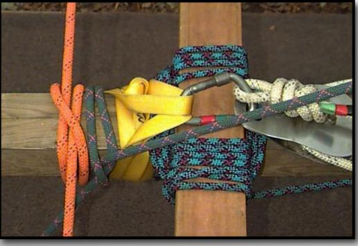
Place the guy lines on the gin pole using 1/2" kernmantle rope.
