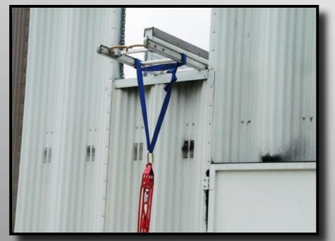
A counterweight at the butt end should be used, such as lashing the butt end to an anchor point, or have two rescuers sit on butt end of ladder.
